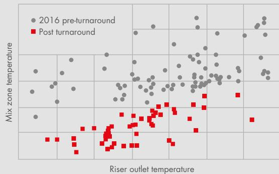
Figure 1: Riser temperature above the mix zone for pre- versus post-turnaround operations.
