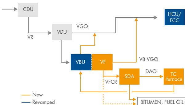
Figure 1: An integrated VDU-VBU-SDA-TC DAO-HCU/FCC line-up. The key is to first maximise the straight-run distillate that is extracted from the vacuum column before treating it first by cracking and then by SDA.
