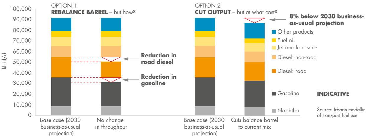
Figure 1: The impact on refiners of changes in road transport. With even modest assumptions about the changes in transport, refiners face a significant mass balance or throughput challenge.
