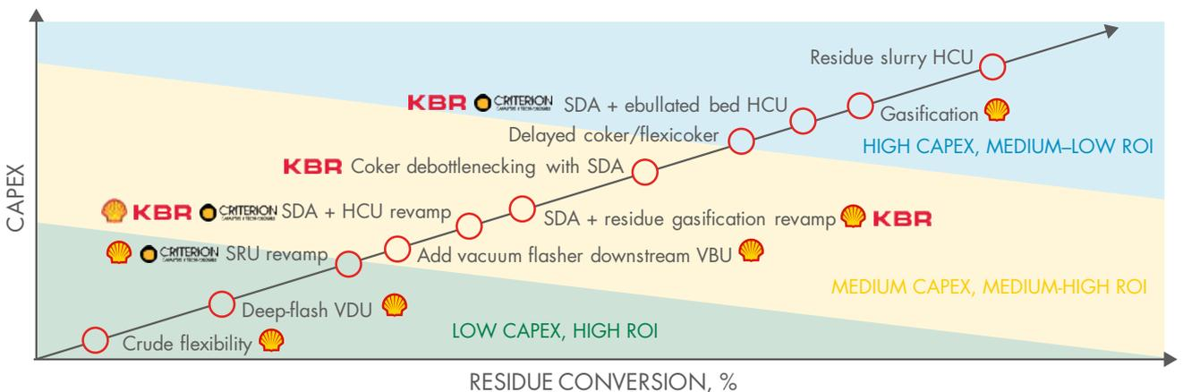
Figure 1: Some of the technology solutions that can help refiners to respond to IMO 2020.
